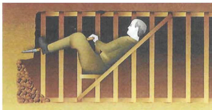
Figure 1. Clay kicking, a tunneling technique from the North-West of England that found application in the trenches in soft rocks and cohesive soils on the Marne front [27].
